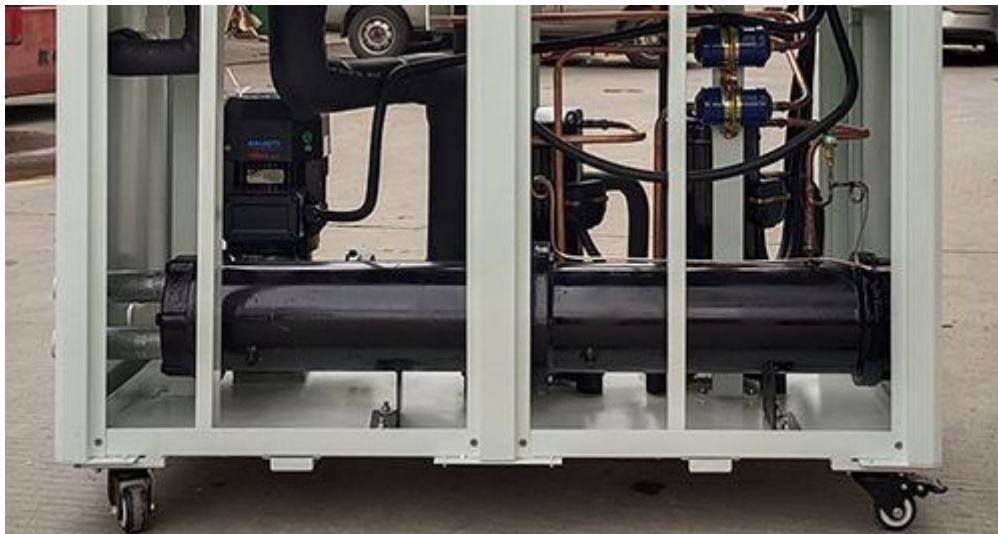
Shell and tube Condenser for water-cooled Anodizing chiller
